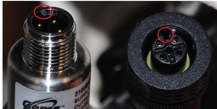
**PRESSURE SENSOR CONNECTION CODING**
