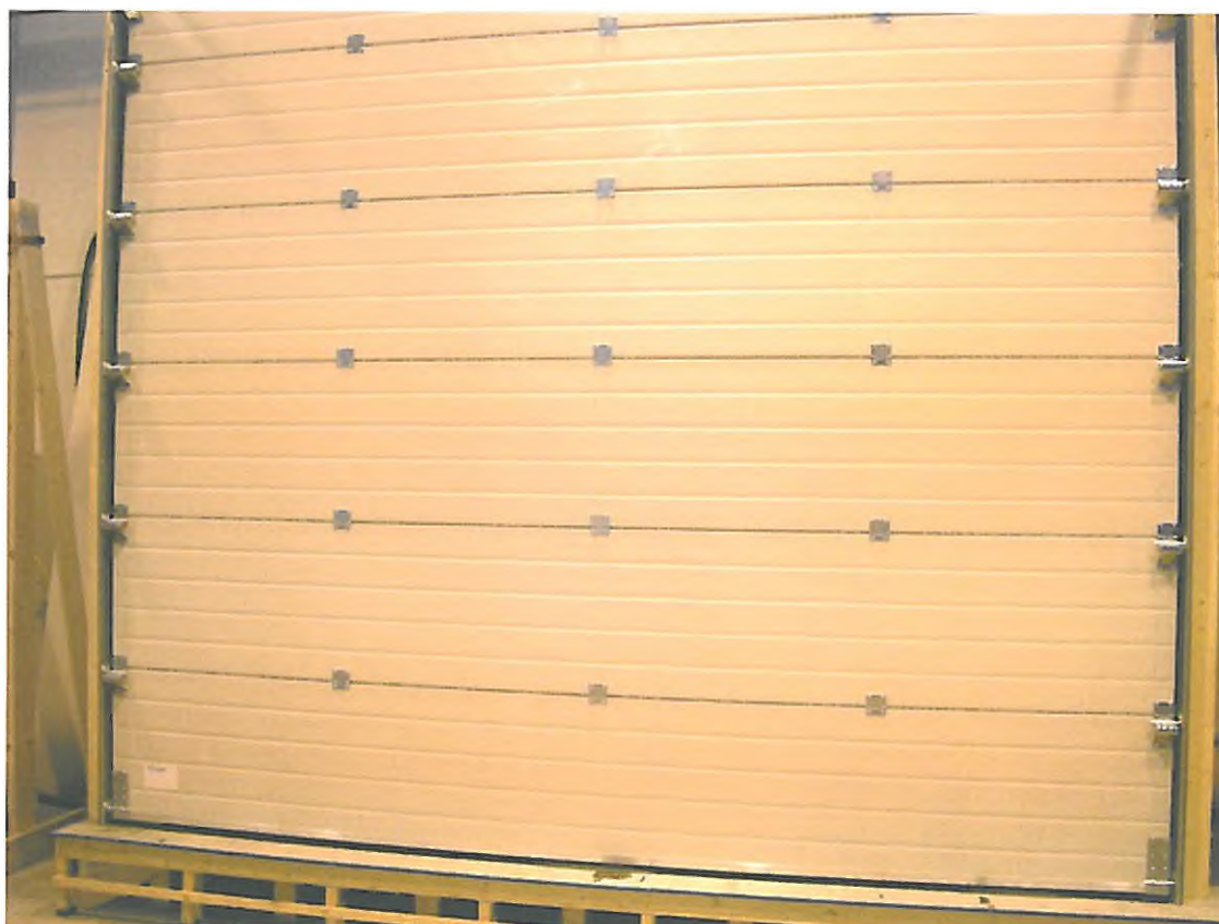
Figure 2. Door type FlexiForce, Standard Lift with Sicom panels mounted in the test rig, as seen from inside.
