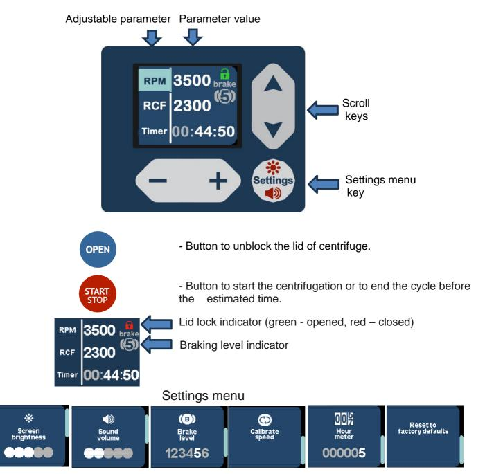
Parameters such as screen brightness, beeper volume and brake level can be adjusted in the settings menu.
