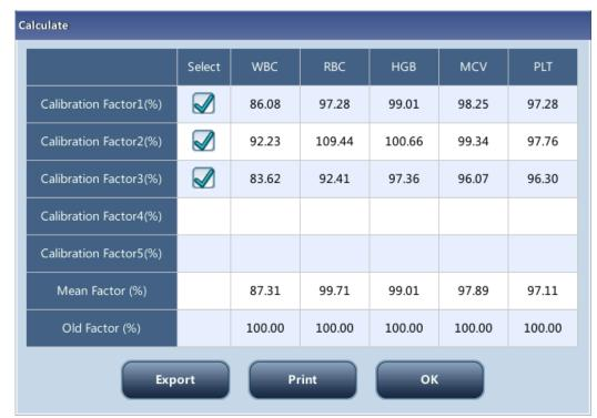
Select or deselect the calibration factors of a blood sample for the calculation of the Mean calibration factors by tapping the check boxes before the calibration factors.
