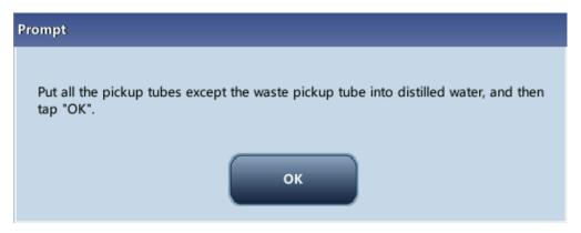
5. Place all reagent pickup tube assemblies into the distilled water, and then tap the "**OK**" button to start priming.
