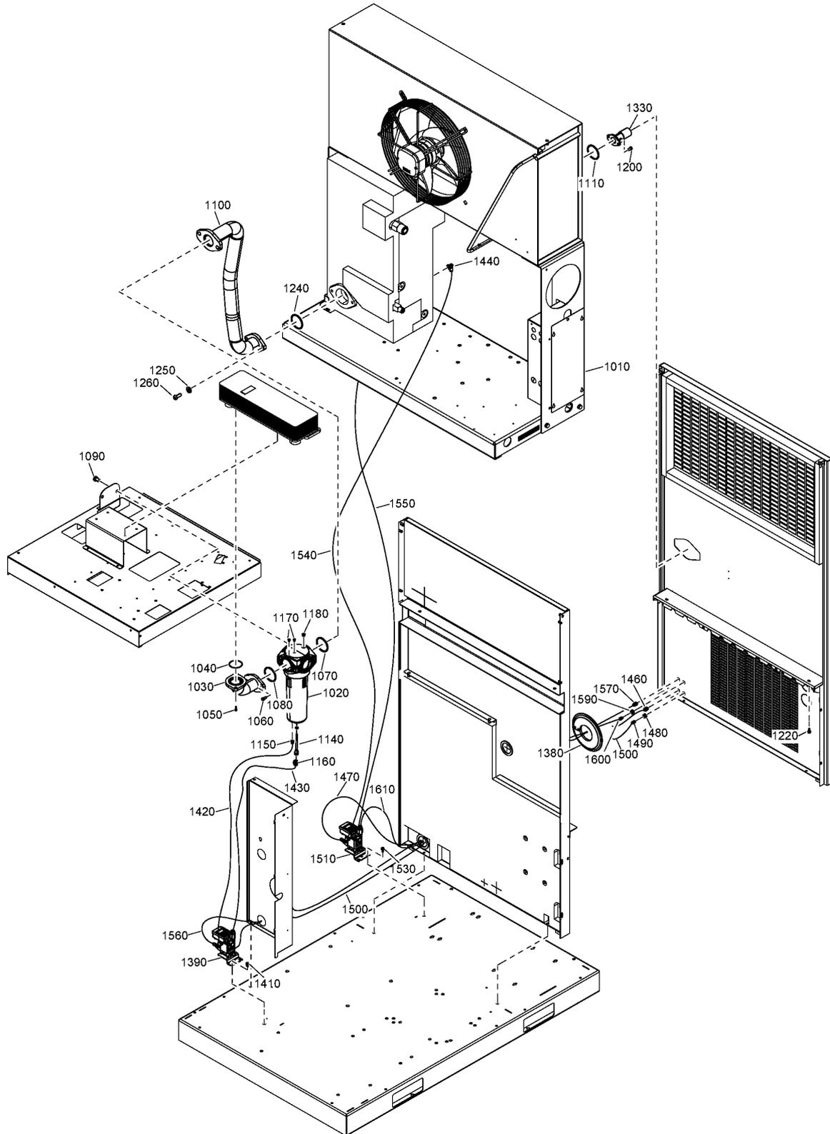
**14 - Air outlet - Water-cooled (GA 37L VSD+, GA 45 VSD+, GA 55 VSD+ - 380V-460V/60Hz, 400V/50Hz), (GA 75 VSD+ - 380V/60Hz, 400V/50Hz) - Full-Feature**
