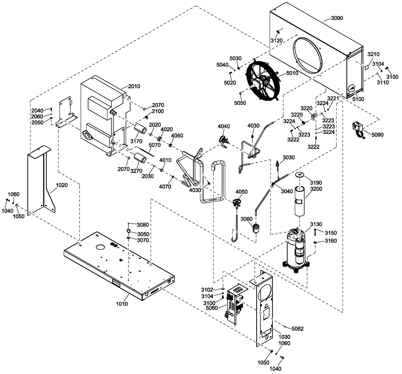
**18.3 - Components GA 37L VSD+, GA 45 VSD+, GA 55 VSD+ - ID180 - 460V/60Hz IEC, 230V-460V/60Hz UL-cUL**
