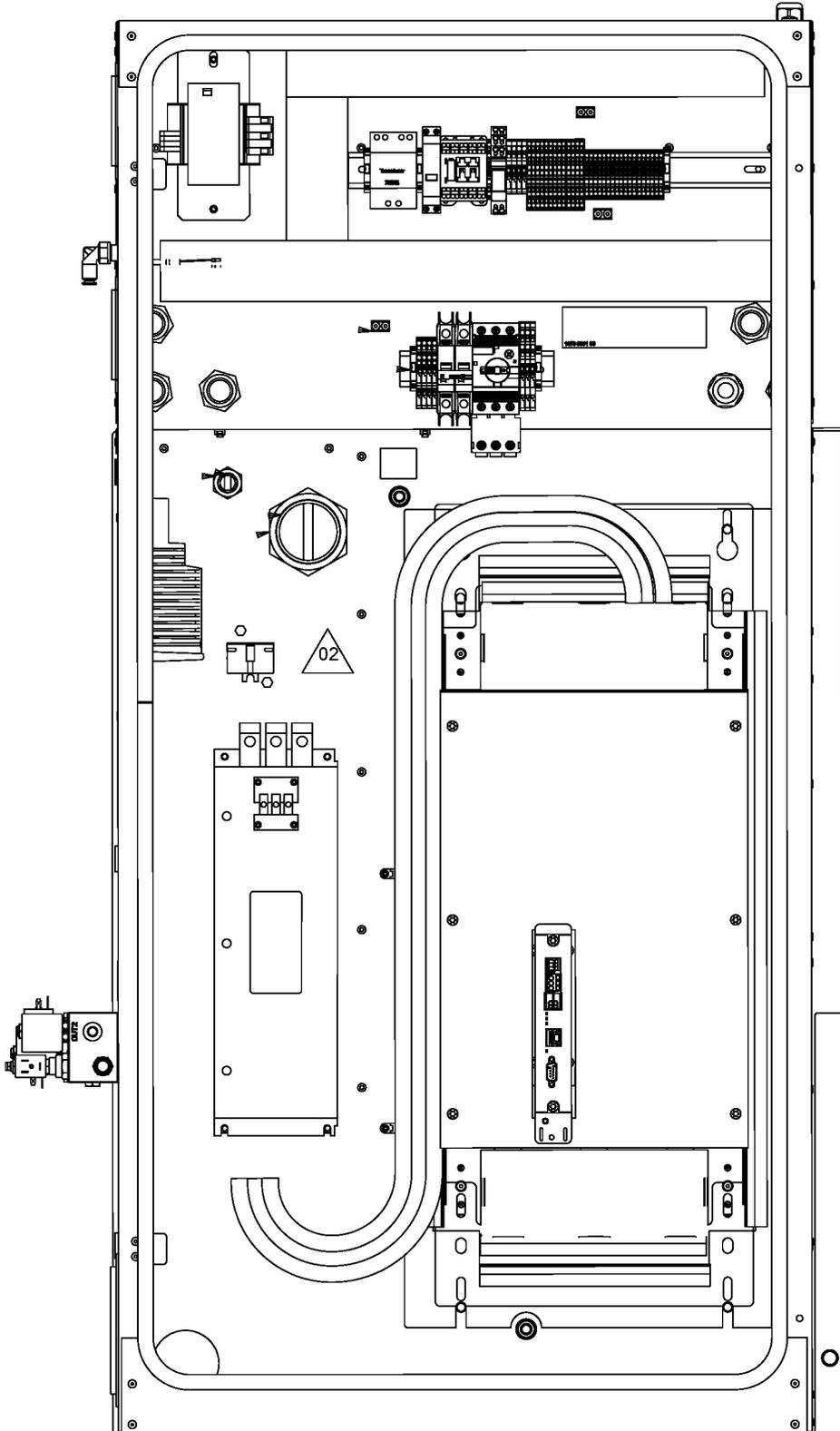
**19.6 - Cubicle components GA 37L VSD+, GA 45 VSD+ - 460V/60HZ (25/07/2019 - 12/02/2020)**
