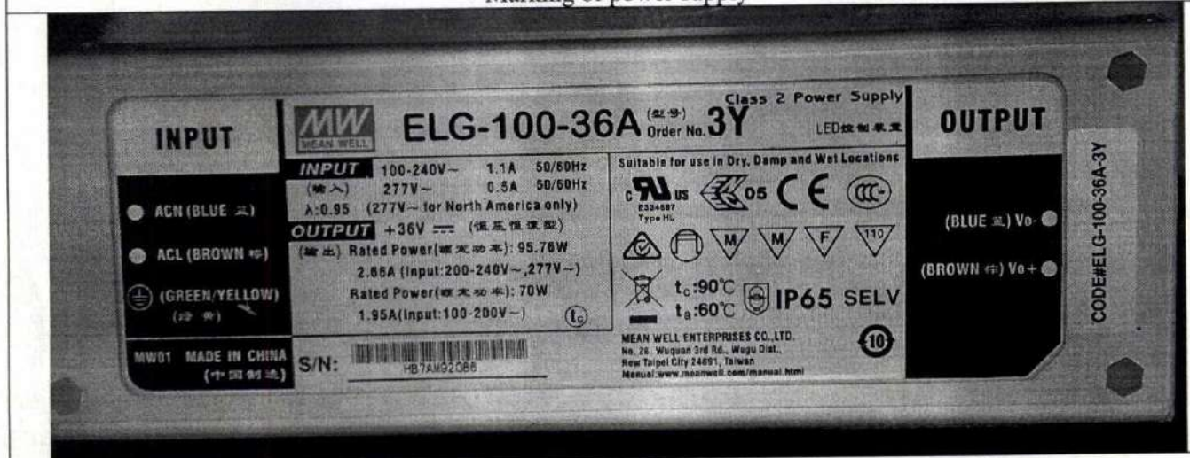
Marking of power supply
