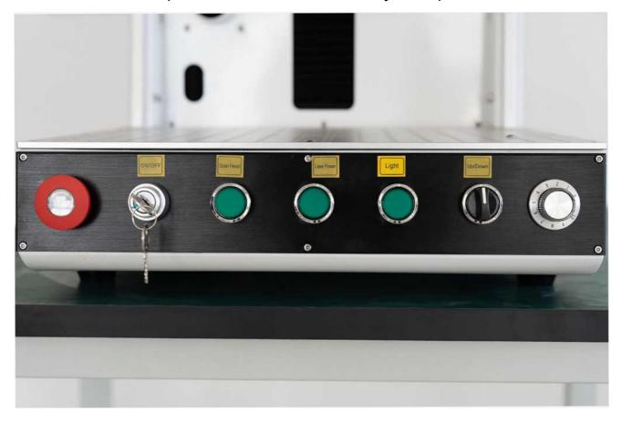
Each major component has an independent control button, galvanometer, lifting and lowering speed can be independently controlled, further improving the working experience of the staff.
