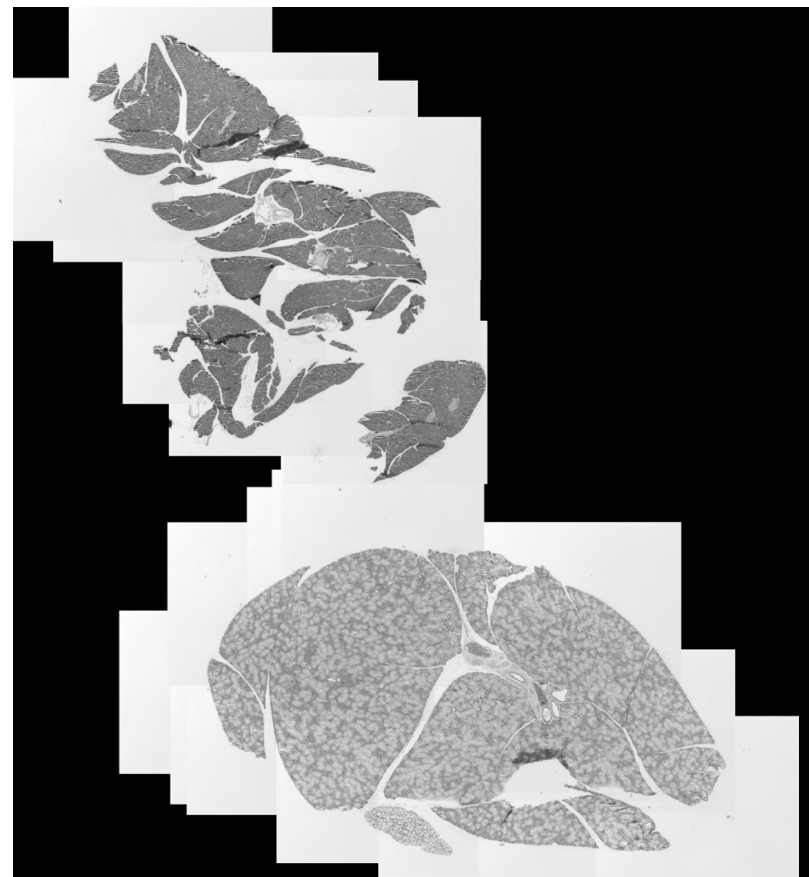
Brightfield images of a tissue section acquired using Live Panorama. ZEN automatically takes images and stitches them, while you manually navigate the area of interest on your sample.
