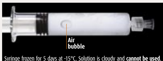
Syringe frozen for 5 days at -15°C. Solution is cloudy and cannot be used.
