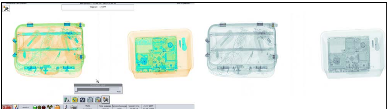
Figure 47 – Display mainly based on high energy data: the highest absorption details are shown, otherwise they would be invisible
