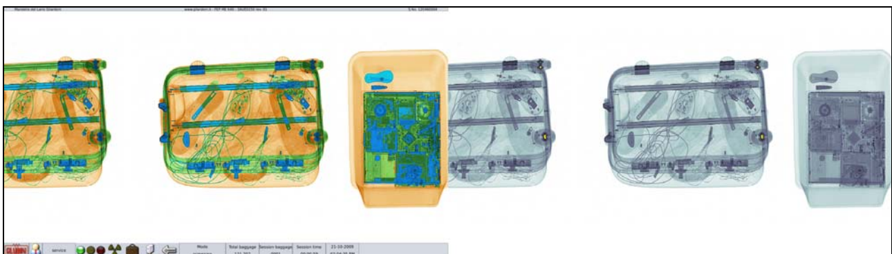
Figure 10 – Typical 2 monitor X-ray image by FEP ME 640: color and grey-scale view
