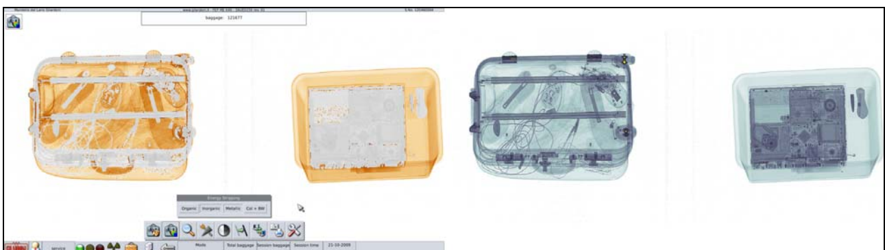
Figure 49 – Energy Stripping: removal of metal and inorganic materials
