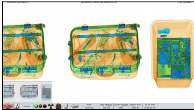
Figure 11 – Typical single monitor X-ray image by FEP ME 640: colour view and grey-scale miniature
