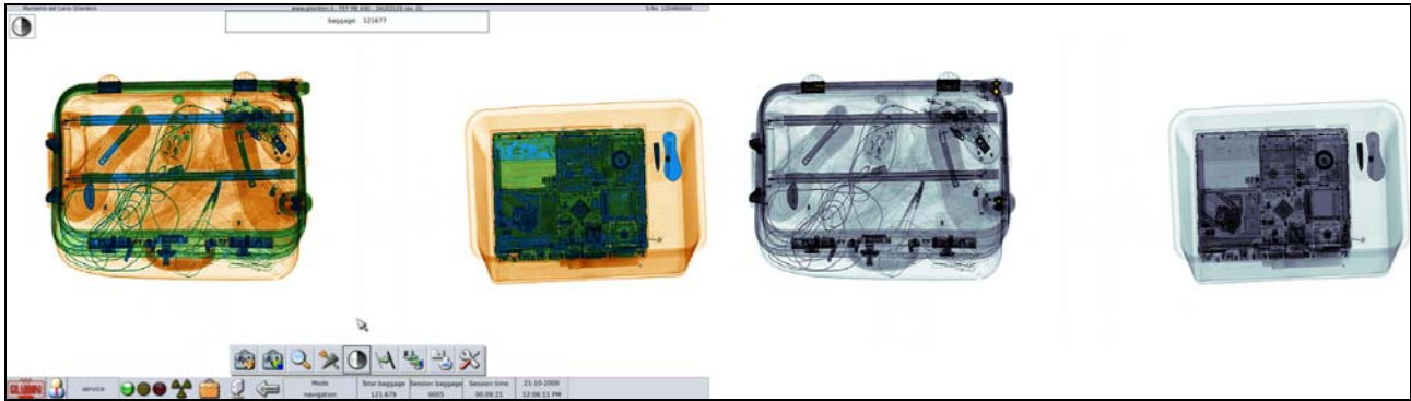
Figure 46 – Strong contrast effect entered by ‘Optimum contrast’
