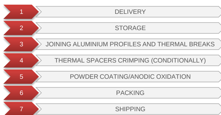
Fig. 3. A scheme of manufacturing of the facade systems by Aluprof S.A. in factory in Bielsko-Biala (Poland).
