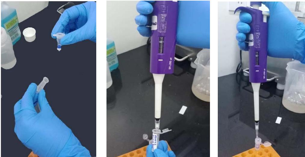
14. Close the tube gently and centrifuge for 1 minute at 8,000 rpm. The eluate in the Micro Centrifugal Tube 1.5ml (PW146) contains pure RNA.
