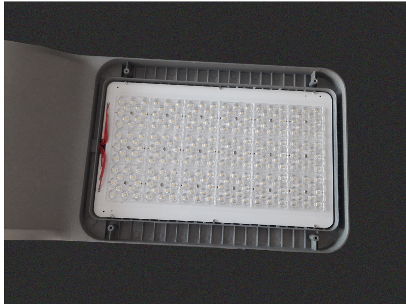
Photo 5 -- After the test of IP65
