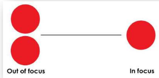
Figure 7.5: Aiming beam focusing
