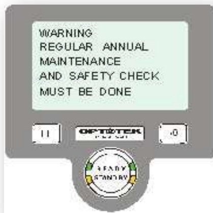
Figure 9.3: Laser maintenance message
