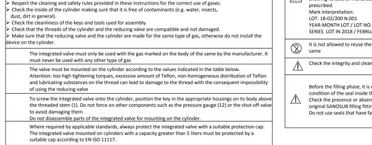
Before the filling phase, it is necessary to remove the filling connector cap (6), check the presence and condition of the seal inside the filling connector cap. If damaged, replace it.
