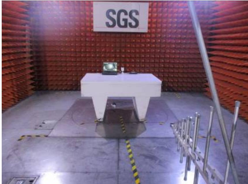
**8.4 Radiated Emissions (above 1GHz) Test Setup**
