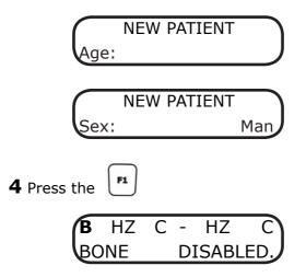
Use the corresponding attenuator to select the application conduction of the signal for each channel: bone  $(\mathbf{O})$  or disabled (-).
