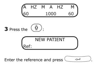
If there are thresholds that have not been saved in the database from the previous patient, the equipment will display the following screen which allows them to be saved:
