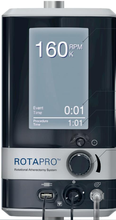
Rotational Speed Display (Tachometer)
