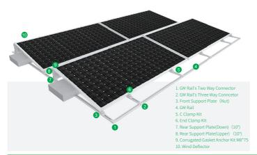
MRac Roof Solar PV Mounting System RM-Ad is a non-penetration solution for flat rooftop, an extension from RMI, to meet different tilt angles installation. It is applicable to the roof areas with medium wind load. Quick installation and stable structure are assured by the modular patented design.
