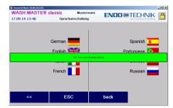
After saving, use the ESC button to return to the setup menu.
