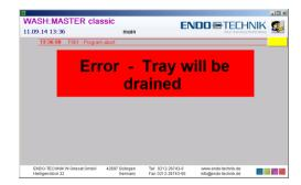
Reset the fault by tapping Acknowl.
