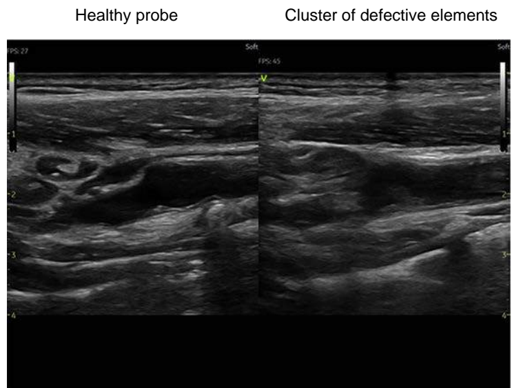
Figure 13-26. Example of image degradation for a linear probe
