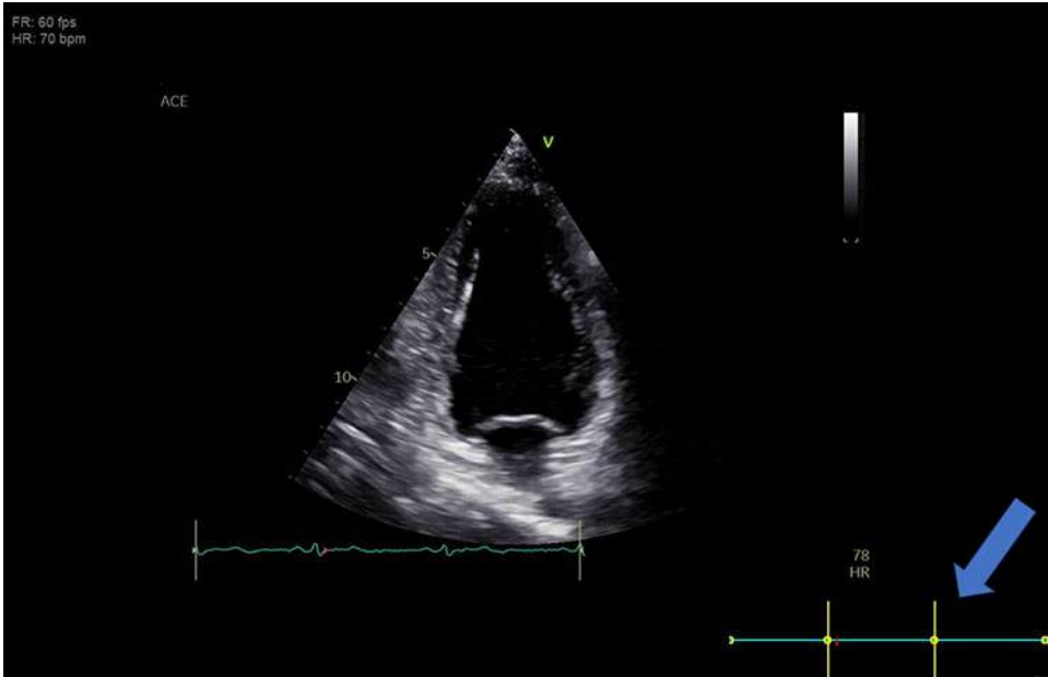
Figure 8-13. ECG representation in AFI when performed on DICOM data. If the required tag was found, cycle starts will be displayed as yellow dots on the ECG line.
