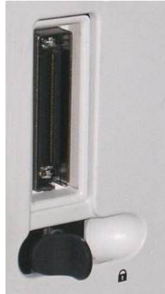
Figure 3-18. RS Probe Connection Locking Lever
