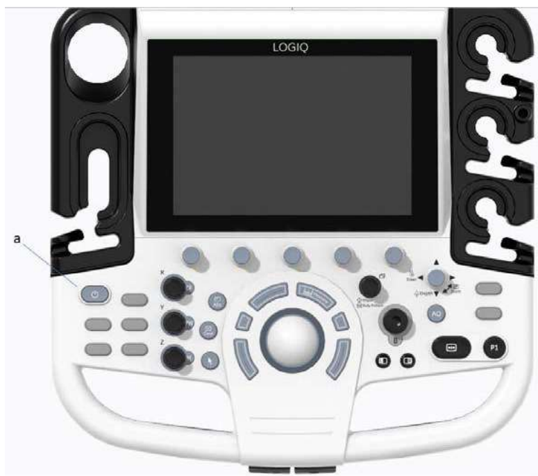
Figure 3-20. Power On/Off Switch Location
