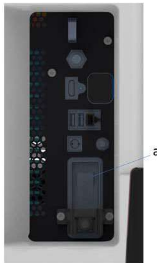
Figure 3-27. Circuit Breaker (located on the rear panel)
