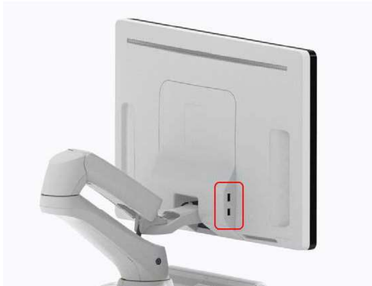
Figure 9-12. USB port on HD Display
