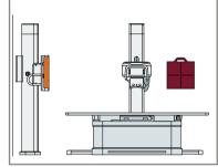
Floor-mounted solution with motorized Bucky wall stand with Core static and fixed table equipped with Core XL for free exams
