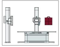
Floor-mounted solution with motorized Bucky wall stand and fixed table equipped with Core XL for free exams
