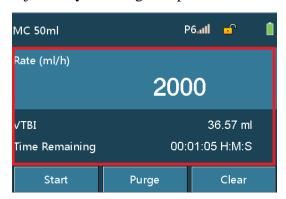
Function button area: Displays such buttons as [Start], [Purge], [Clear], [Stop], and [Bolus]. Setting buttons such as numbers and letters appear on corresponding interfaces.
