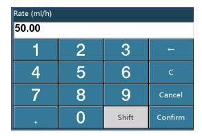
• After entering the rate and tapping [Confirm], the system returns to the original infusion interface and operates at the new rate; if you tap [Cancel], the system returns to the original infusion interface without change.
