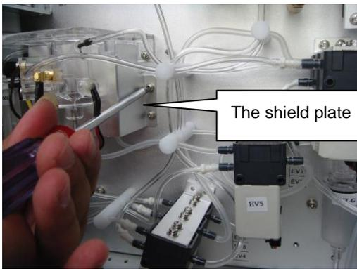
2. Remove the three fixed screws of counting chamber
