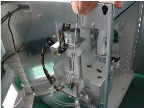
5. Remove tube of sample probe.
