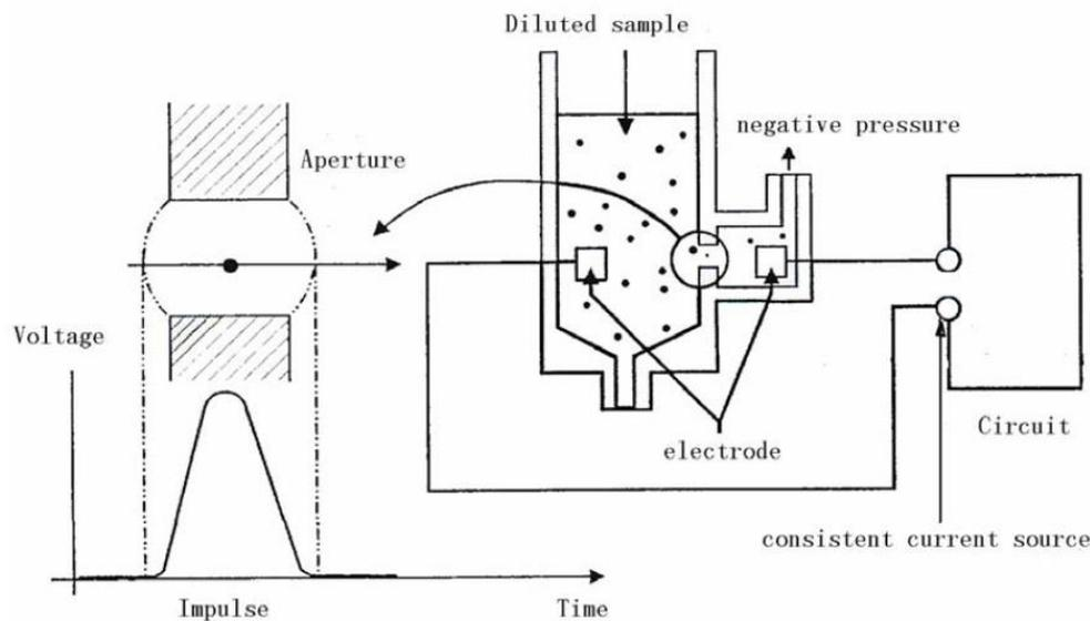
Figure: Impedance Method of Counting and Sizing
