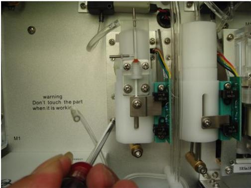
3. Remove signal cable connector from main controller board.
