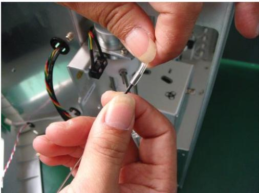
Note: it is a little difficult to remove this tube from sample probe, it is very tight,
