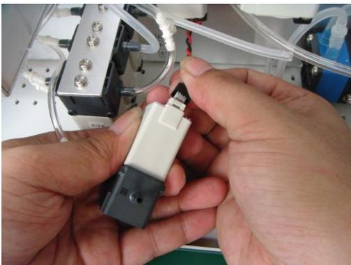
5. Remove the two fixed screws to open valve.
