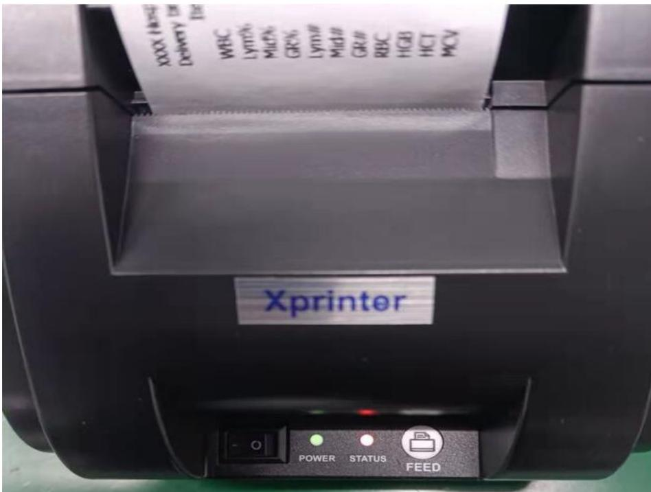
5. When switch on the printer, the green light is always lighting. And if paper is detected by printer, the red light is always lighting also, otherwise red light is flickering.
