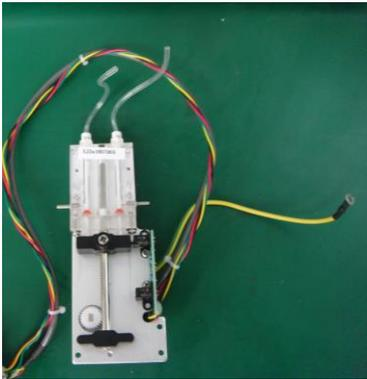
8. Remove the four fixed screws of syringe cavity.
