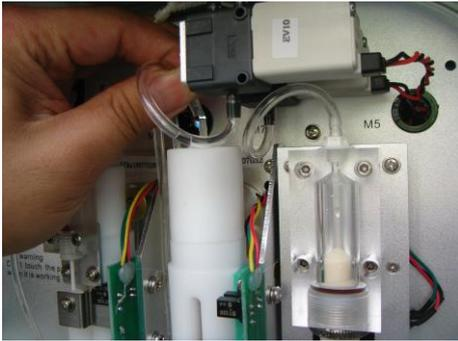
3. Remove the three fixed screws of subassembly.
