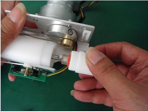
10. Reverse above steps to install new O-ring of lyse syringe.
