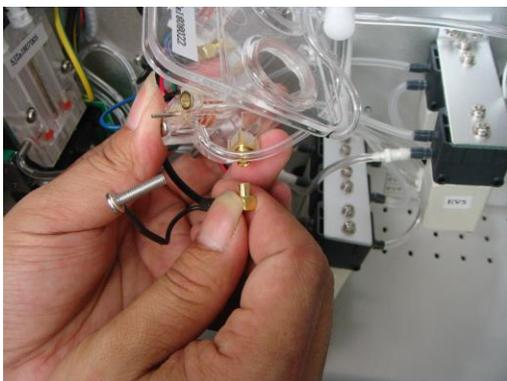
4. Remove two tubes which are connecting with backseat of aperture.
