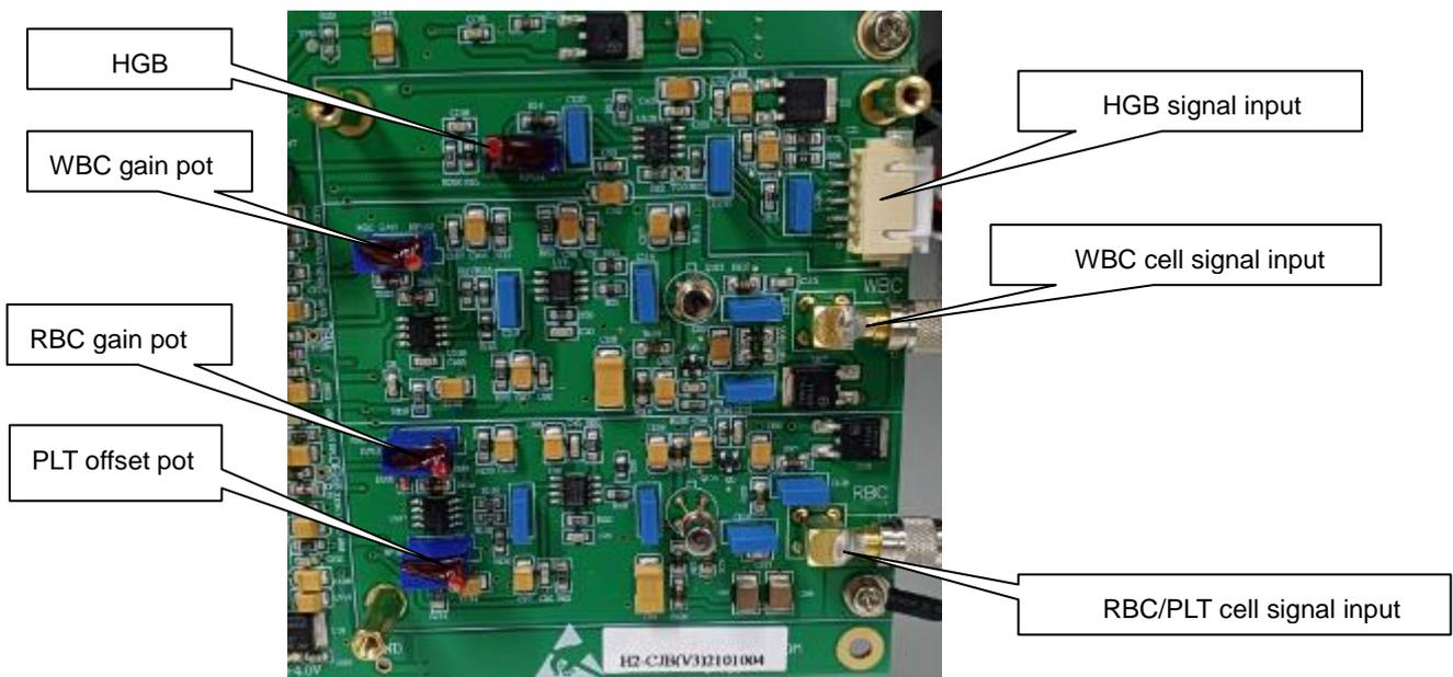
Note: U102 (L78M18) and U103(L78M18) transform DC24V to DC 18V for WBC and RBC channel cell count.
