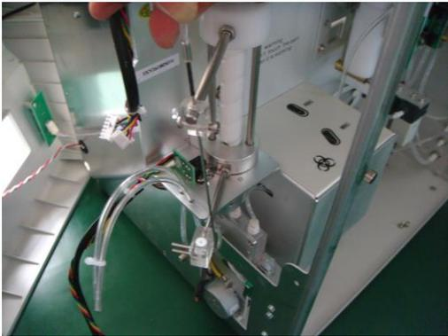
5. Remove two fixed screws of subassembly and then can remove the whole subassembly.
