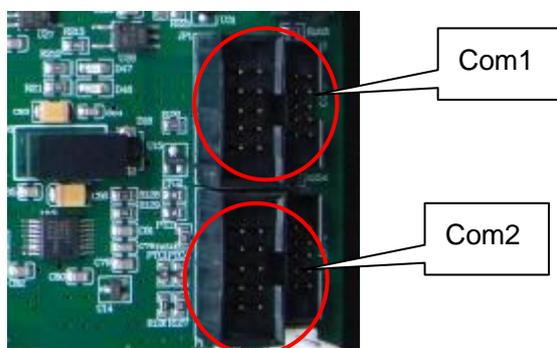
Com1 is connecting with com1 of ARM main board. It is used to communicate between analyzer software with main controller board.
