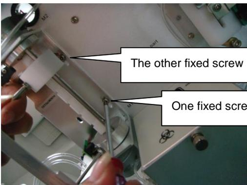
6. Reverse above steps to install new sample probe subassembly.
