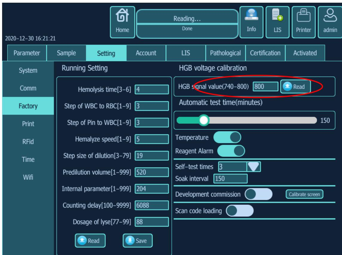
Step 3, if this signal value is not in the range, we need to replace the HGB lamp or it photocell.
