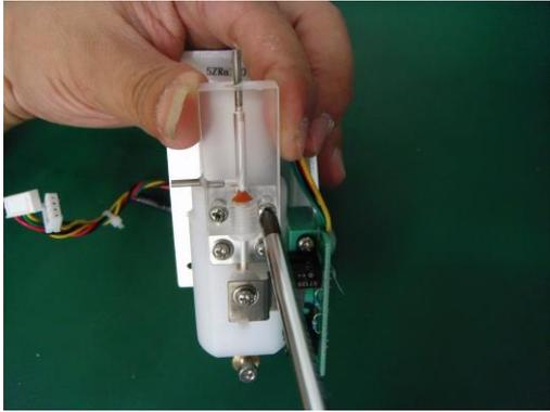
6. Pull out the sample syringe cavity.
