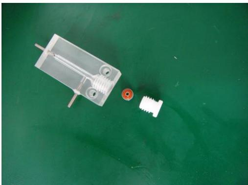
8. Reverse above steps to install new O-ring of sample syringe.
