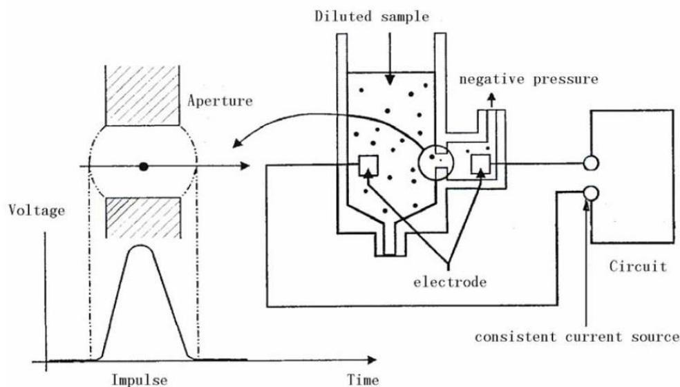
Figure: Impedance Method of Counting and Sizing
