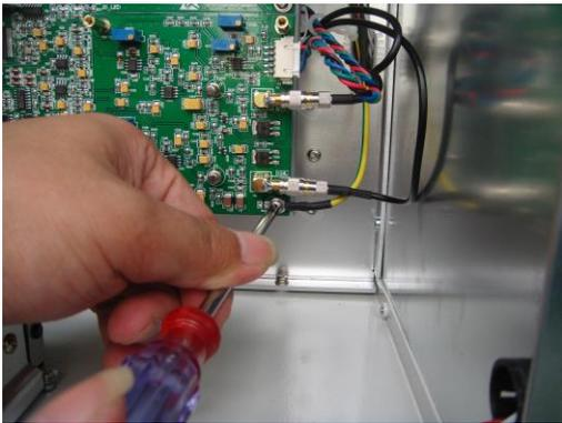
5. Remove signal cable connectors from main controller board.
