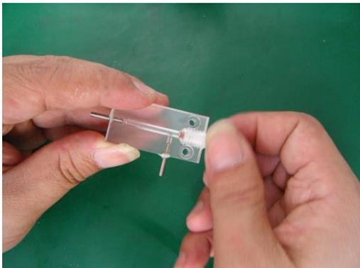
7. Unscrew the fixed screw of O-ring.
