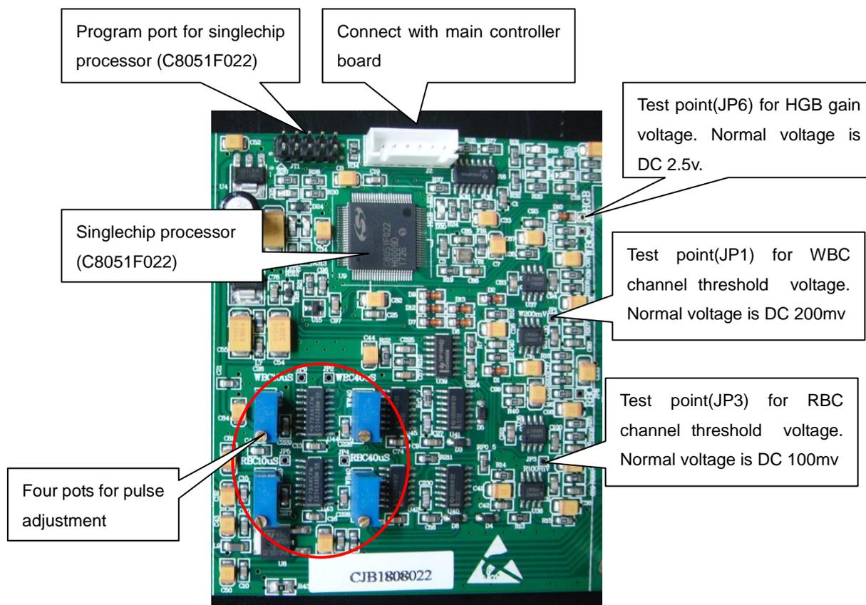
**Note: Potentiometer of WW10,WW40,WR10,WR40 are used to adjust WBC and RBC channel pulse, they are only adjusted by factory engineer using oscillography, otherwise it is very difficult to adjust for service engineer and customers.**
