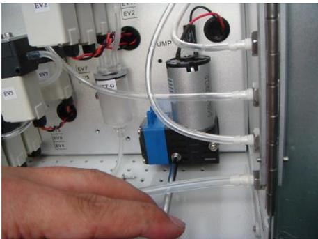
3. Remove the four fixed screws of membrane cover.
