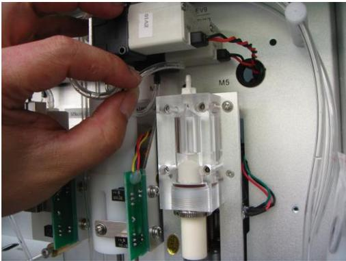
3. Remove the four fixed screws of subassembly.
