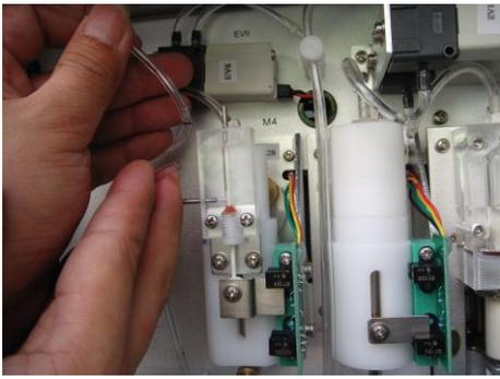
2. Remove the three fixed screws of subassembly.
