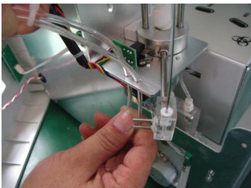
3. Remove signal cable connectors of sample probe subassembly from main controller board.
