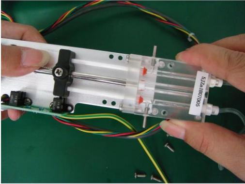
10. Remove the two fixed screws of O-ring block.
