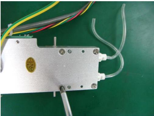
9. Pull the syringe cavity out.
