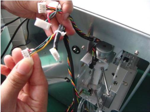
4. Pull out sample probe from washing head.
