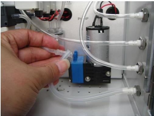
2. Remove the two fixed screws of waste pump.
