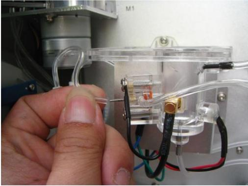
4. Remove ground connector of syringe from data process board.
