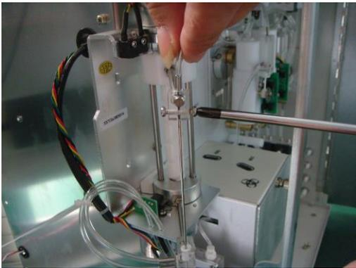
4. Pull sample probe out of washing head.
