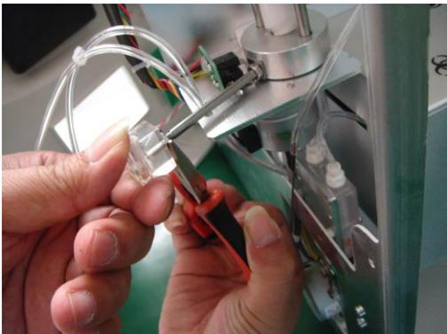
4. Rotate washing head and then can remove it.
