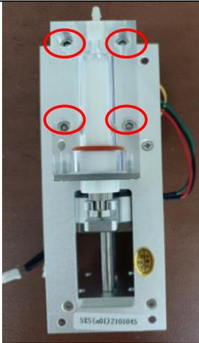
5. Remove the four screws and pull out the piston from the diluent syringe cavity.
