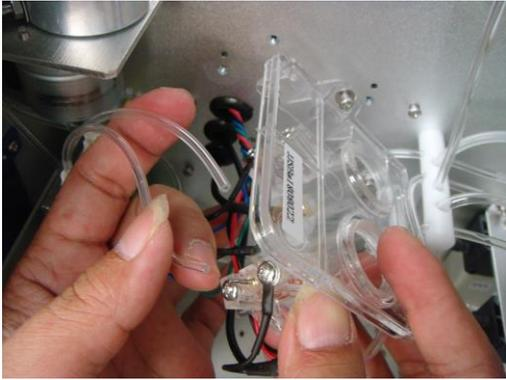
5. Unplug electrode cable from data process board.
