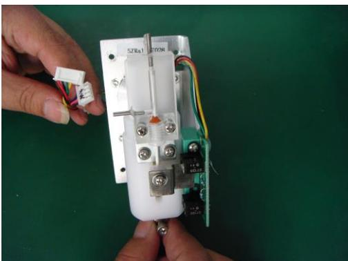
5. Remove the two fixed screws of sample syringe.
