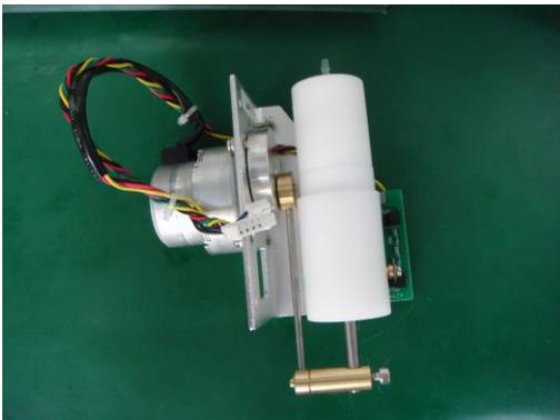
5. Rotate detergent syringe cavity and then can remove syringe cavity.
