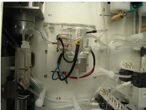
3. Remove the four tubes from counting syringe.
