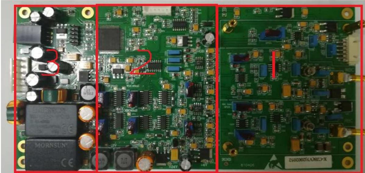
The data process board consists of three modules according function.
