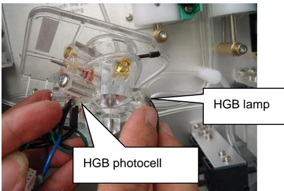
3. Pull out the HGB lamp and HGB photocell from counting chamber.
