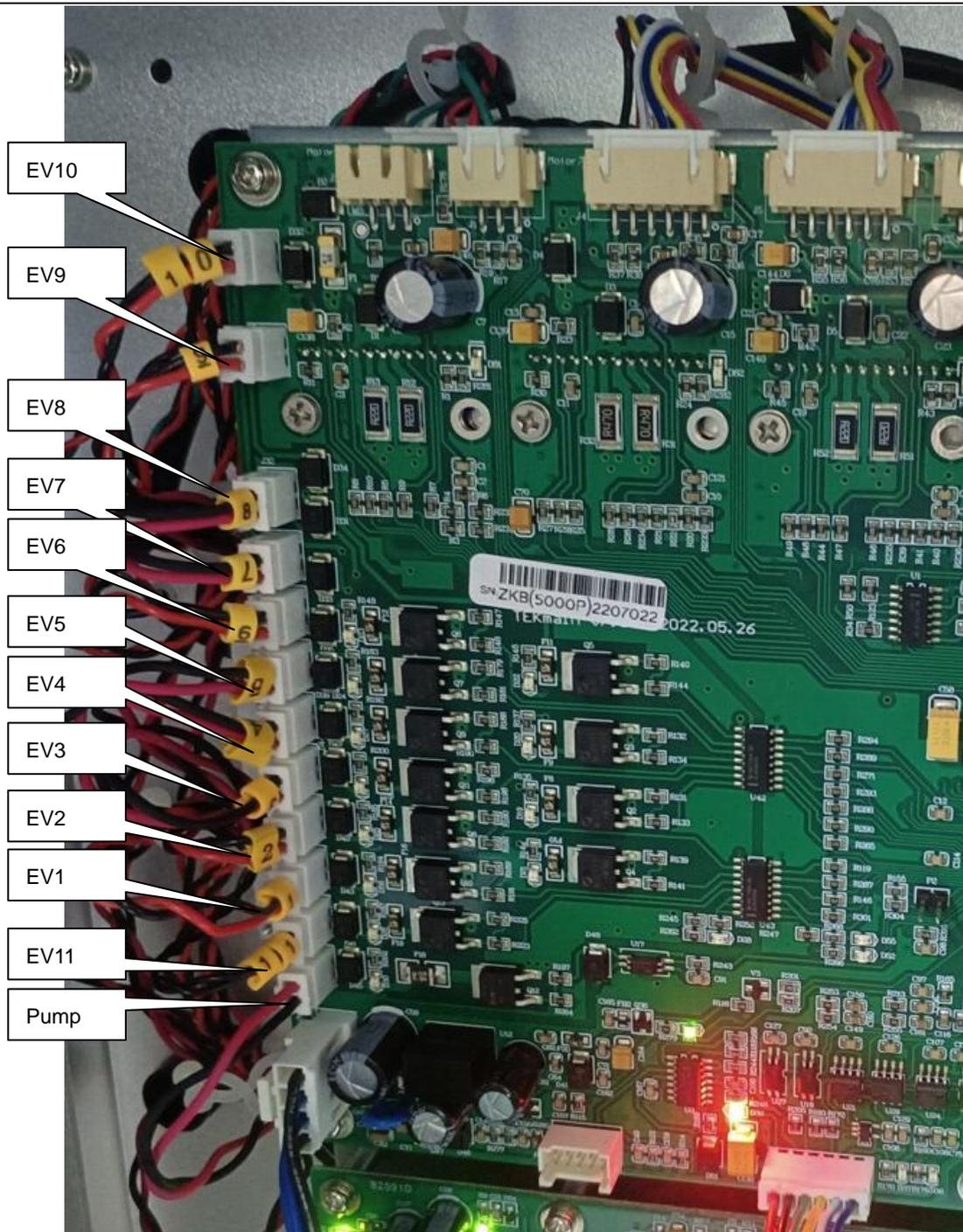
Note: pump and EV connectors must connect with the according sockets that name marked on the board. Different version board the sockets positions may be different.
