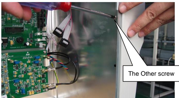
2. Lift up the front panel and then pull outward.
