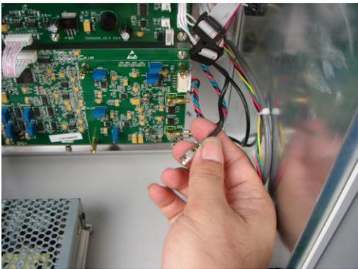
6. Reverse above steps to install new electrode cable.
