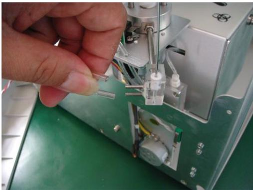
2. Pull out the two tubes from assembly holes.
