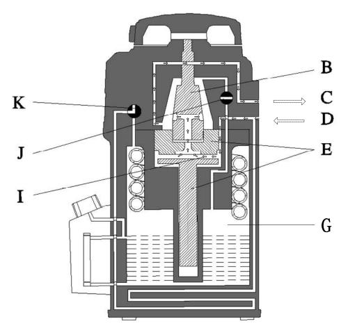
Fresh gas flows from the inlet D to the airway I, and then passes the temperature compensator E and the cone valve B, finally flows out from the outlet C.
