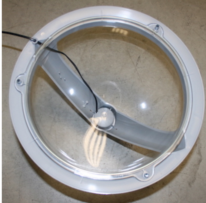
Photograph No. 15 Optical diffuser, with supply cable 2 x 1 mm 2 H05RN-F
