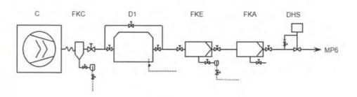
C: KAESER oil cooled screw compressor FKC: liquid separator D1: KAESER refrigeration dryer FKE: KAESER micro filter KE FKA: KAESER activated carbon filter KA DHS: air main charging system
