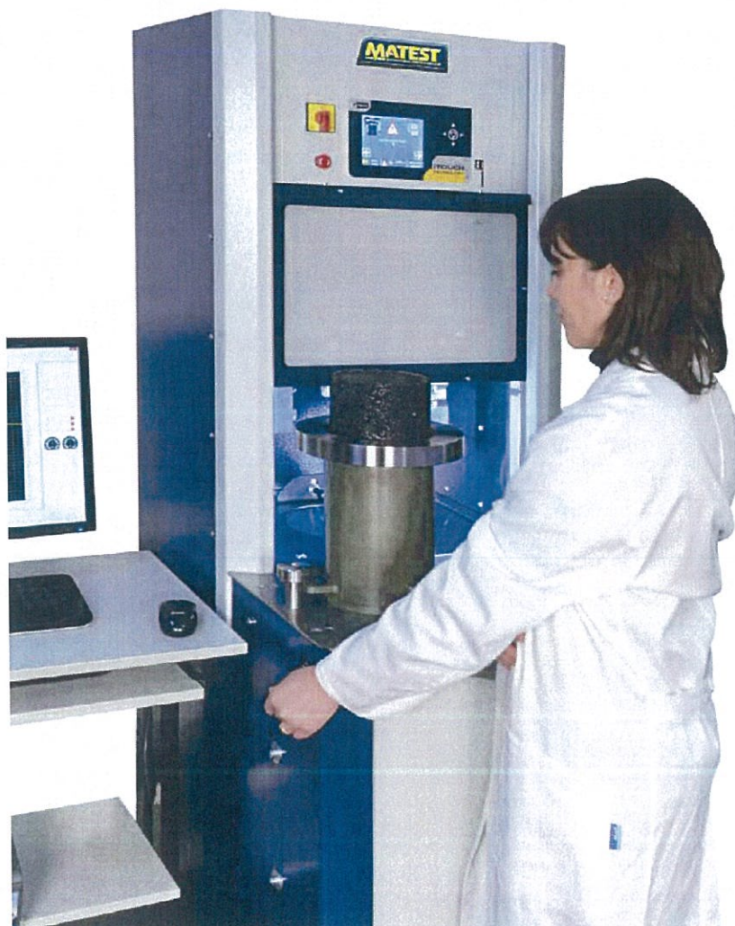
Test execution with shear stress measurement
