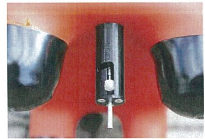
Surface thermometer integrated on the underside of the measuring case
