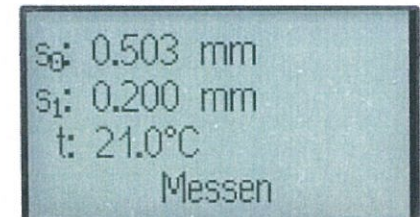
Display of the dual-gauge Benkelman Beam during measurement
