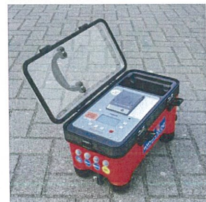
Measuring case of the dual-gauge Benkelman Beam
