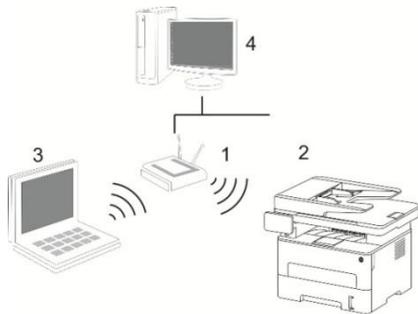
Basic structure mode: connecting to a wireless device via router
