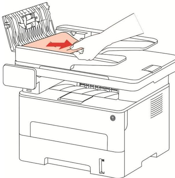
3. After removing the paper jammed, close the top cover and then the printer will be back to the ready state.
