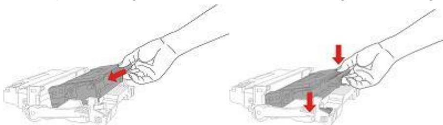
7. Take the drum component with toner cartridge installed and install it inside the printer along the inner track of printer to finish installing.
