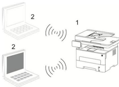
Wi-Fi Direct mode: wireless client is connecting to a printer with Wi-Fi function
