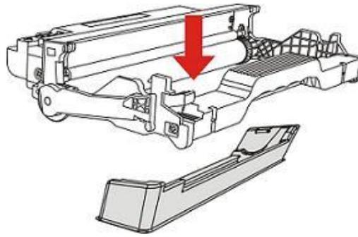
5. Install the drum component along the inner track to finish installing toner cartridge.
