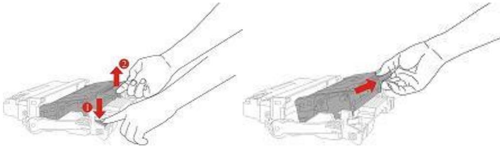
4. Open the package of new drum component, take the protection device of drum component, and put the drum component on a horizontal table.
