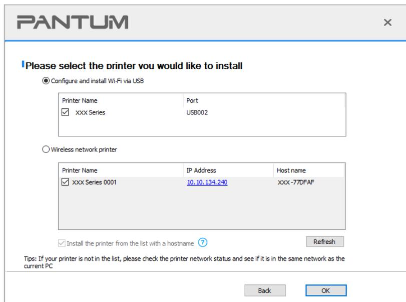
**Note:** When the printer IP address changes under printer driver installed with host ID, you can also directly print without re-installing the driver. If you need to install the printer driver with the host ID, please check the option "Install the printer in the list with host ID".
