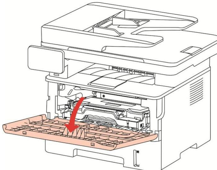
5. Take the laser toner cartridge out along the track. (For the purpose of preventing printing quality from affecting by the exposure of photosensitive drum, please put the laser toner cartridge inside the protection bag or wrap it with thick paper).
