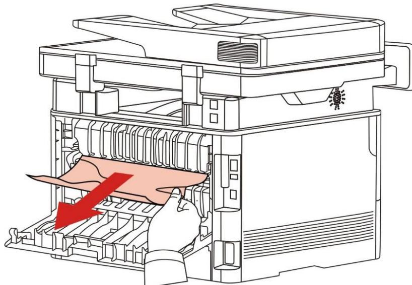
5. Close the back cover after removing the paper jammed.
