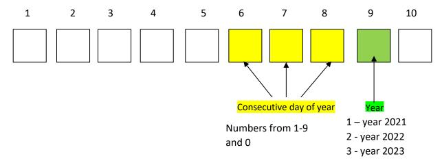
E.g.: 6BAII 1533K means that the battery was manufactured (153 – day, 3 – 2023) on 8th of June 2023.
