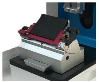
The orientation of the samples is possible in a simple and precise; if the red lights are visible, then the guidance plan is in zero position. The steel clamp is equipped with a device to "clamp" for quick change of the sample and sample holder fixed tilt.
