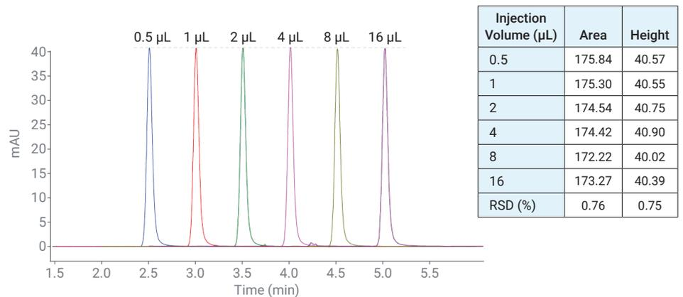
**Figure 4.** Injection volume linearity measurements using caffeine.
