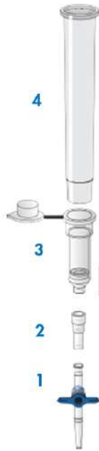
Figure 4. Assembly of QIAamp Mini columns with extension tubes (for buccal swabs or large volumes).
