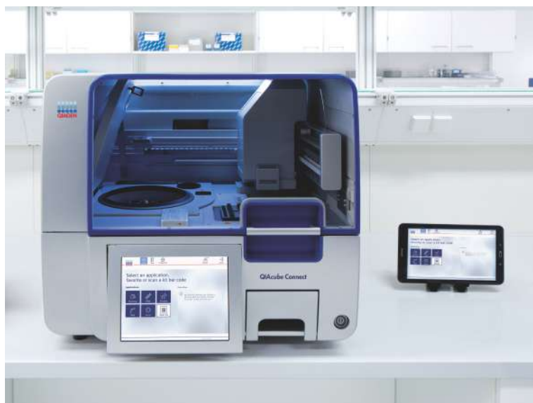
Figure 1. Automated DNA purification. DNA purification using the QIAamp DNA Mini Kit or the QIAamp DNA Blood Mini Kit can be fully automated on the QIAcube.
