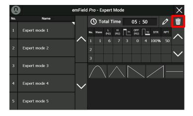
To remove a sub-mode, press the bin figure in the right top corner after choosing the specific sub-mode.
