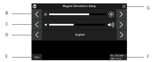
(B) Brightness(C) VolumeAdjust the brightness by using the left and right arrows.Adjust the volume by using left and right arrows.
