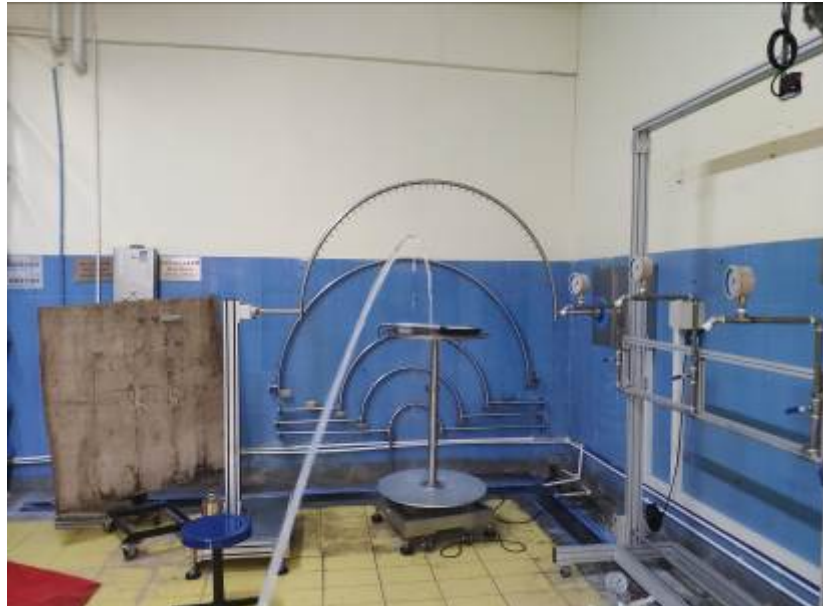
Photo 4 -- During the test of IPX5
