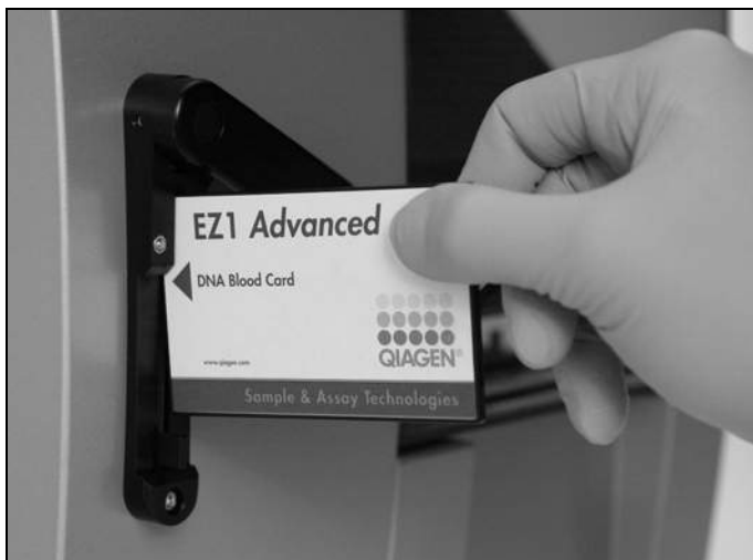
Figure 7. Ease of protocol setup using EZ1 DSP Cards. Inserting an EZ1 Card, containing protocol, into the EZ1 instrument.
