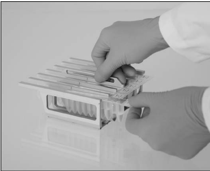
Figure 9. Ease of instrument setup using reagent cartridges (RCB). A A sealed, prefilled reagent cartridge (RCB) of the EZ1 DSP DNA Blood Kit. B Loading reagent cartridges (RCB) into the cartridge rack. The cartridge rack itself is labeled with an arrow to indicate the direction in which reagent cartridges (RCB) must be loaded.
