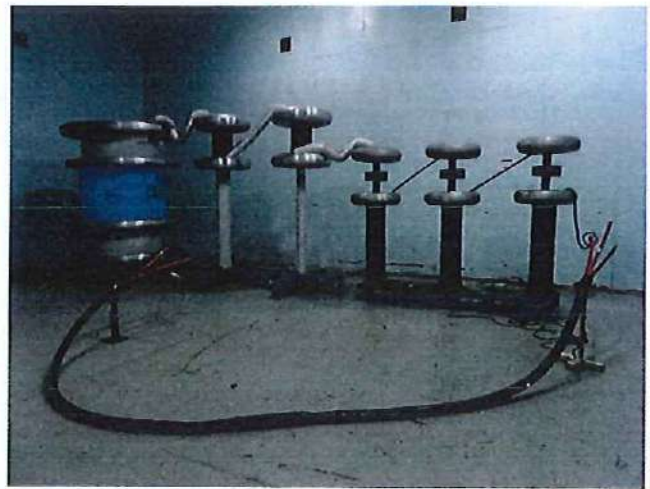
E2: 样品局部放电试验及交流耐压试验 Partial discharge test and AC voltage test on the sample
