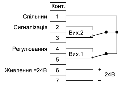
Fig. 1. Contacts of the 2PM18 connector (or similar) in the BP-10B2A
