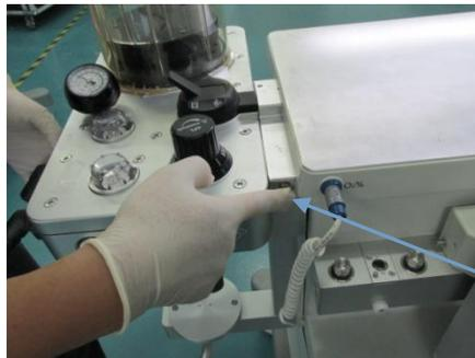
—Take down the circuit on the base seat of the circuit.
