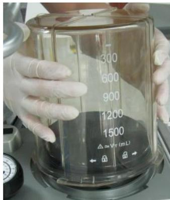
—— Remove the folding bag from the base seat of the bellows.
