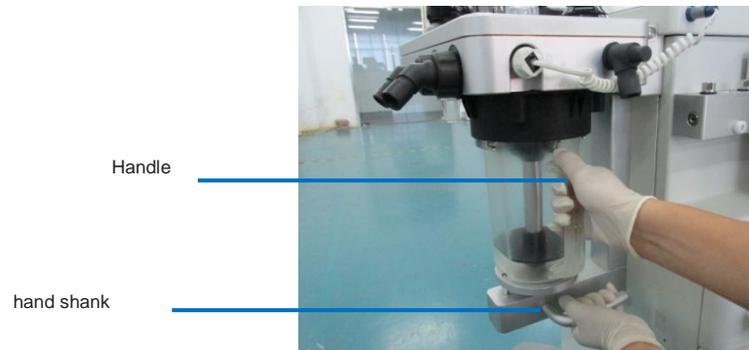
—Guide groove disengage and remove the canister.
