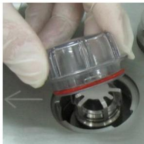
—Pull out the inspiratory check valve from the circuit
