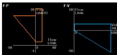
—Lung function ring graph is divided into【F-P】(Flow rate - pressure ring)、【F-V】(Flow rate - volume loop) and【P-V】(Pressure- volume loop. Click in the acyclic graph area, expand the prompt menu, select the desired observation acyclic graph, click【Save Loop】button.
