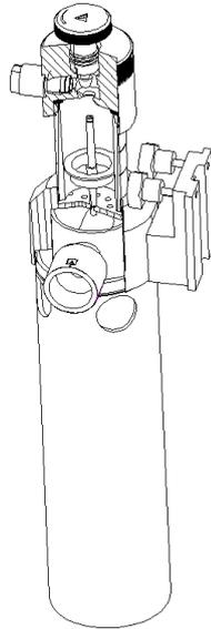
—Counterclockwise unscrew the cover till it is released from the observation window.
