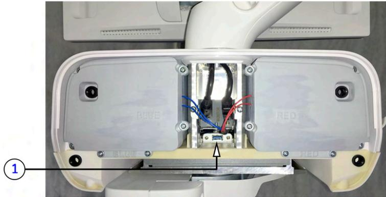
**Note** *This USB port is located inside the Rear Cover Top of the monitor arm. Please remove the cover carefully.*
