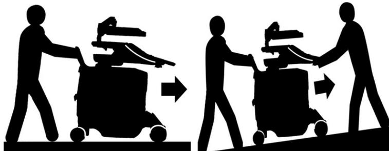
Figure 2-1 Moving the system on plains and inclines
