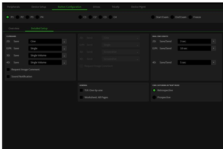
1. **Overview.** Select the basic actions to be performed when pressing a particular P - key.
