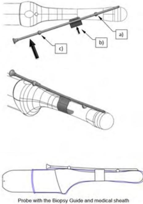
How to adjust the biopsy guide on probes like i.e. RAB6D,.....:
