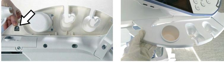
Figure 2-8 Removal of the basic version of the left and right Probe Holder inserts. For installation, just push them back on the user interface until you hear a "click" noise.
