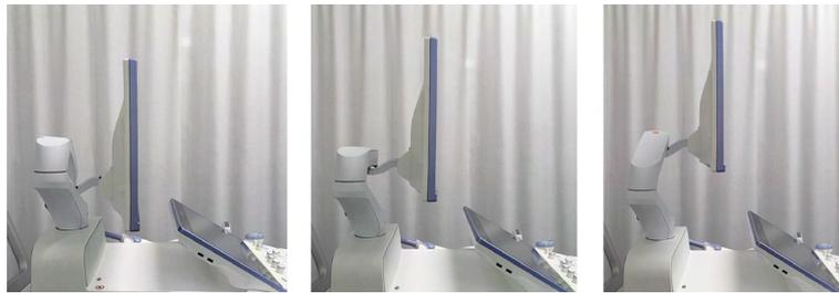
Figure 3-5 Adjusting the height of the monitor.
