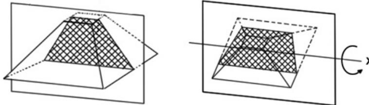
While turning a rotary control, the corresponding axis is shown in the reference image as a line (X- or Y-axis) or as a circle (Z-axis). Rotations around any one of the axes X, Y and Z can be performed freely.
