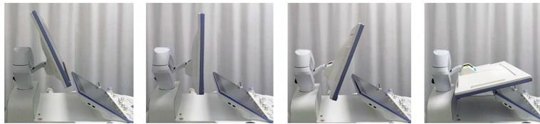
Figure 3-6 Adjusting the inclination of the monitor.
