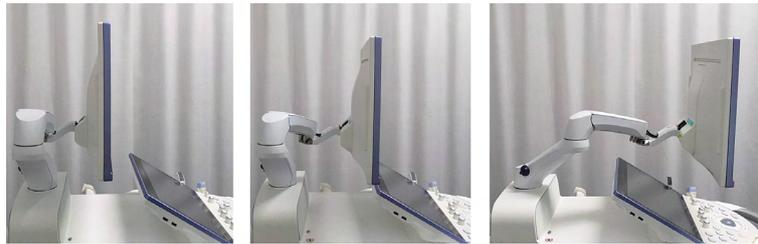
Figure 2-2 Adjusting the monitor back and forth.
