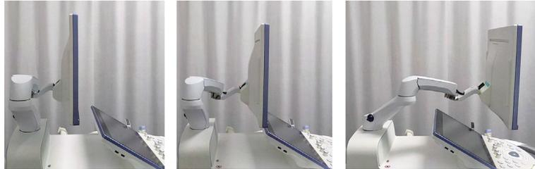
Figure 3-4 Adjusting the monitor back and forth.
