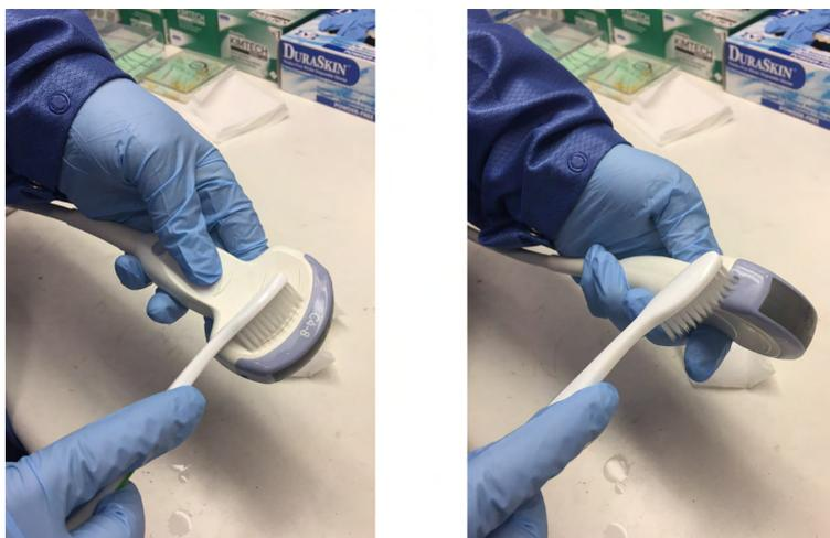
Figure 5-3 Cleaning the probe using a brush
