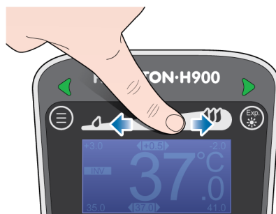
Figure 12. Adjusting Temperature gradient
