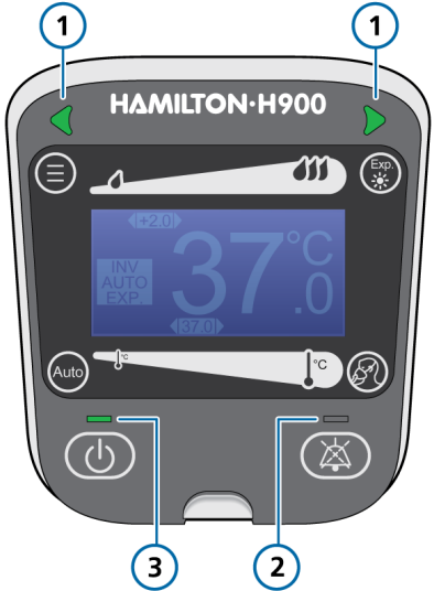
Figure 4. HAMILTON-H900 humidifier, front panel status indicators
