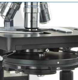
Zernike phase contrast condenser with filter holder
