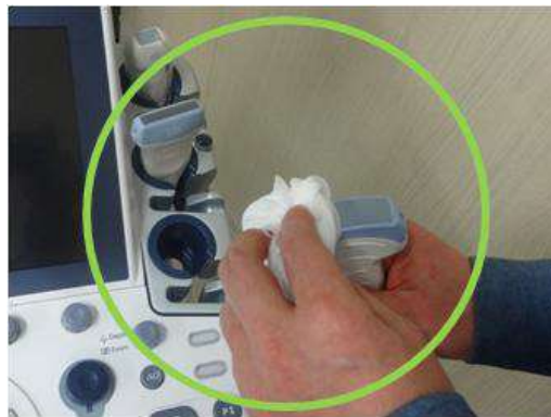
Figure 12-9. Using a Wipe to Clean/Disinfect a Probe
