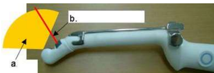
Figure 11-4. Scan plane orientation
