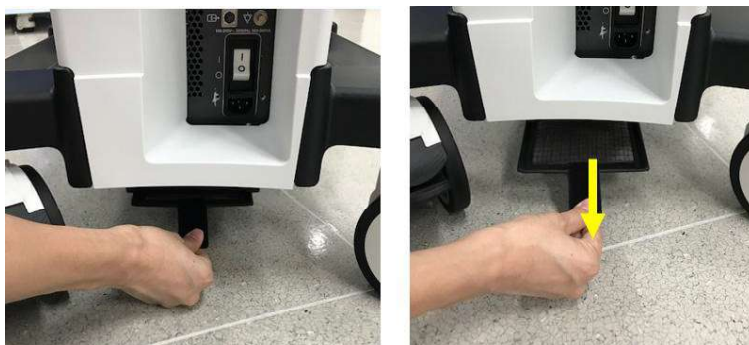
Figure 12-6. Air filter location
