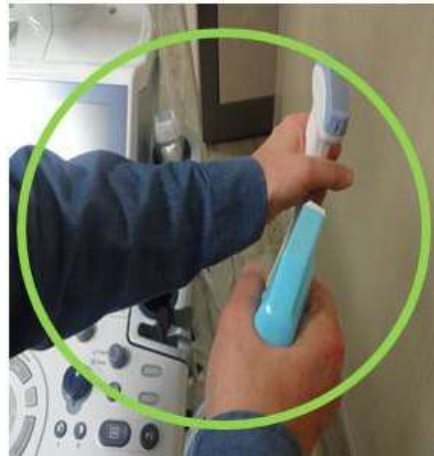
Figure 12-8. Spray Probes AWAY from the Ultrasound System
