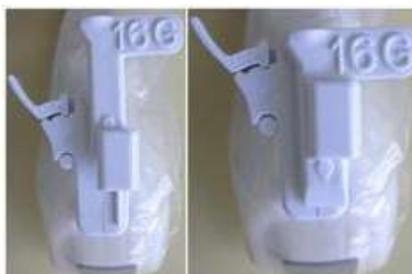
Figure 11-17. Needle Barrel Installation
