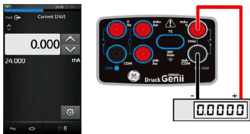
Figure 2-18 Source current on CH2 with internal loop power. (Range: 0 to 24\text{mA} )
