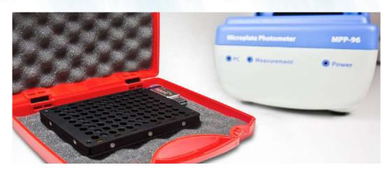
**OD Plate** is the measurement verification instrument for microplate photometer MPP-96 HiPo. The instrument is designed to verify the accuracy and precision of measurements of the photometer at six levels of nominal optical density: 0.3; 0.6; 1.0; 2.0; 3.0; 4.0 OD. The instrument is supplied with the following verification wavelength range: 405-700 nm.
