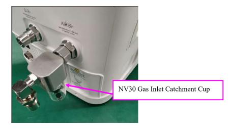
2. Pull the filter out of the NV30 gas inlet catchment cup for replacement.
