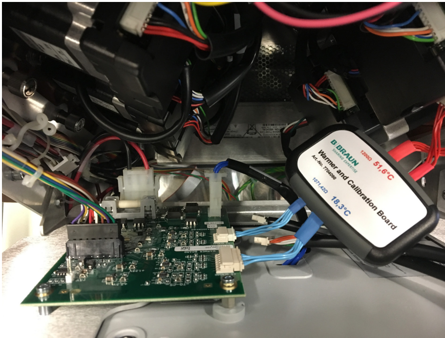
Fig. 1-13 Connection of the warmer test and calibration board to the previous warmer board
