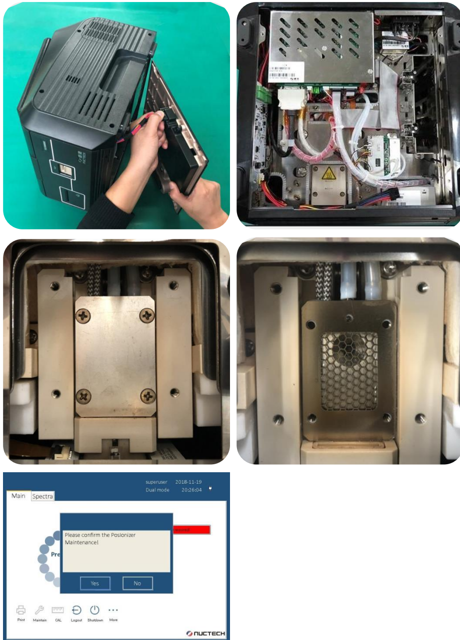
Figure 6.14 Changing the membrane
