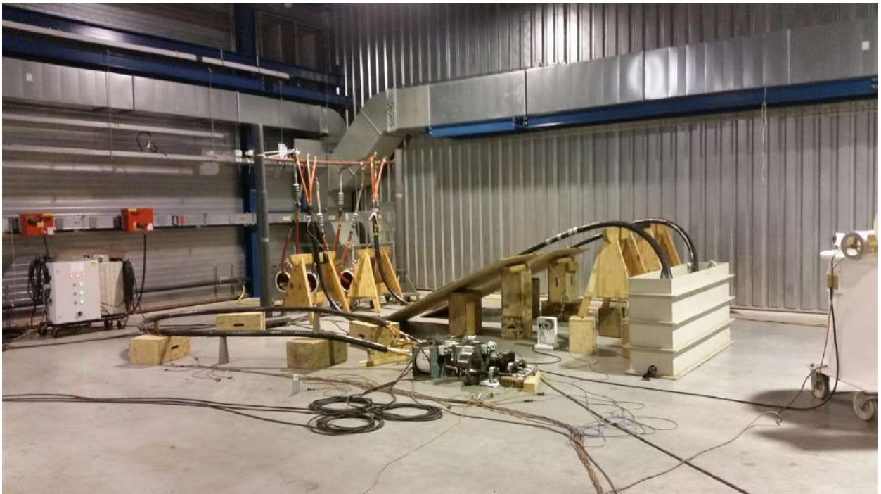
Test set up outdoor termination in immersion test 10 cycles
