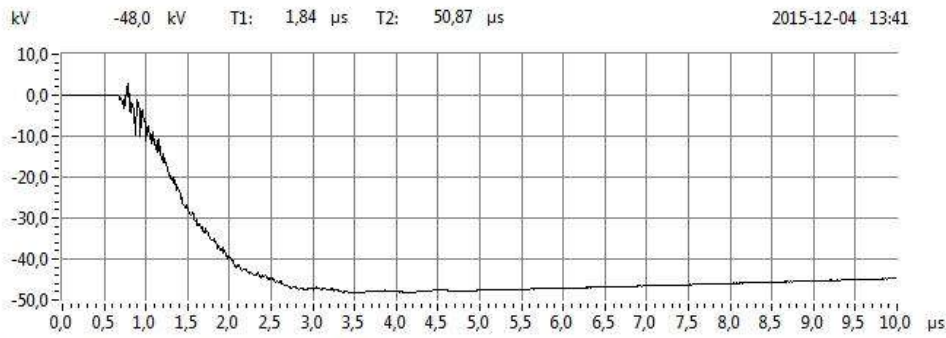
Fig. 5: Waveshape 72124900 SC loop Red -50% test voltage
