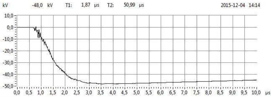
Fig. 13: Waveshape 72124900 SC loop Yellow -50% test voltage
